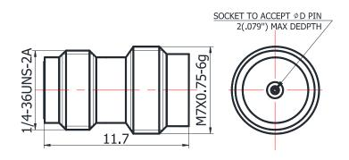
For glass-bead of 0.30mm pin diameter
