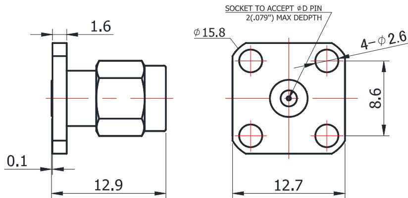
For glass-bead of 0.30mm pin diameter
