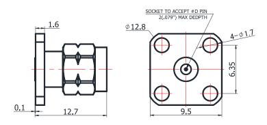
For glass-bead of 0.30mm pin diameter
